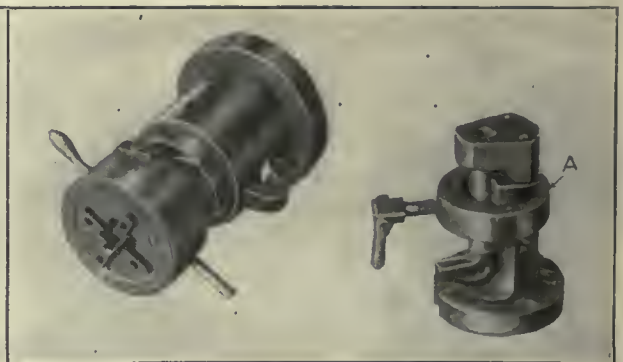
FIG. 4. DIE HEAD USED AS A MILL, AND A DRILLING JIG
